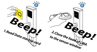
For collect lock events, the light flash will be and it last for 35sec till finished.
